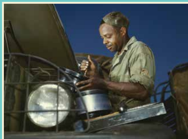
A good job in the air cleaner of an army truck, Fort Knox, Kentucky Photographer: Alfred T. Palmer Library of Congress Prints and Photographs Division www.loc.gov/pictures/item/lsa1992001099/PP
